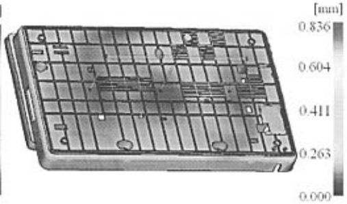
图4.4.3 塑件收缩不均匀引起的翘曲变形量 Fig 4.4.3 Deflection of differential shrinkage
