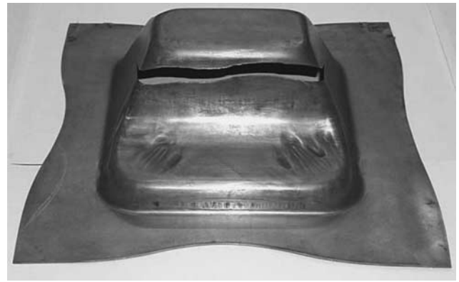
Fig. 7. Split and wrinkles in the production part.
