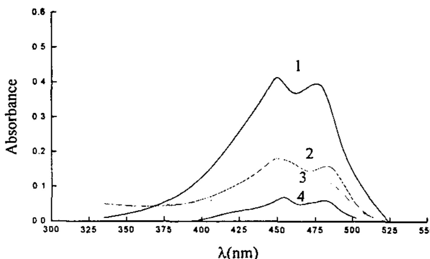
Fig2-4 UV absorption spectra of polyesters and fluorescein
