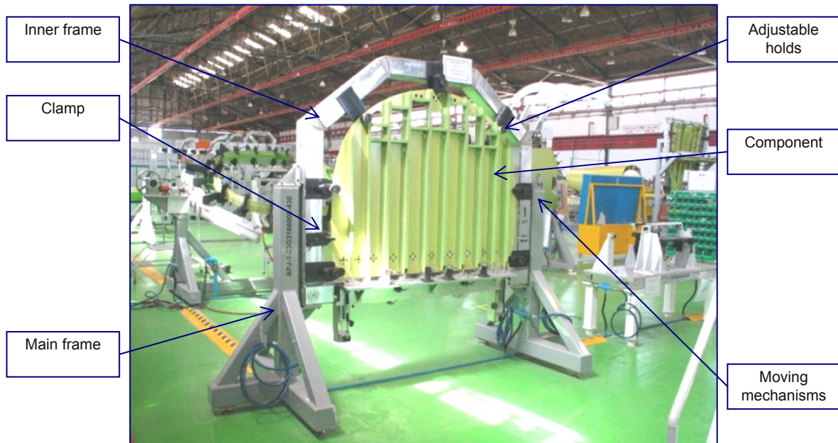
Figure 1: Typical components of large scale jig (image courtesy of Electroimpact http://www.electroimpact.com/G150TFIX/gallery.asp )
