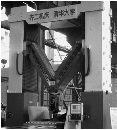
Fig. 7 XNZD2415 hybrid machine tool
