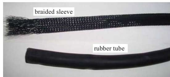
Figure 2. Rubber tube and braided sleeve
