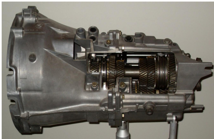
Fig. 2. View of 5-speed gearbox for automotive transmission.
